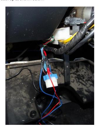
Next find a suitable earthing point on the vehicle chassis for the remaining black wire from the relay box, if you look underneath the steering column there is a single bolt with an E marked on it, loosen this bolt off with a 12mm spanner/socket, remove sufficient insulation from the black wire and slip the wire around the bolt and re-tighten, lastly re-fit the wiring harness back into the correct socket for the ignition barrel.
