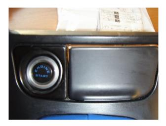
On the reverse side fix the inside part of the button to the outer part using the glue provided, ensure the button is correctly orientated before gluing as the japanese glue provided is extremely strong and sets very quickly.
