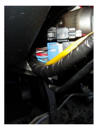
Ensuring the battery is disconnected, remove the socket and free the wiring from the plastic conduit by un-clipping the retaining clips to make it easier to work with.
