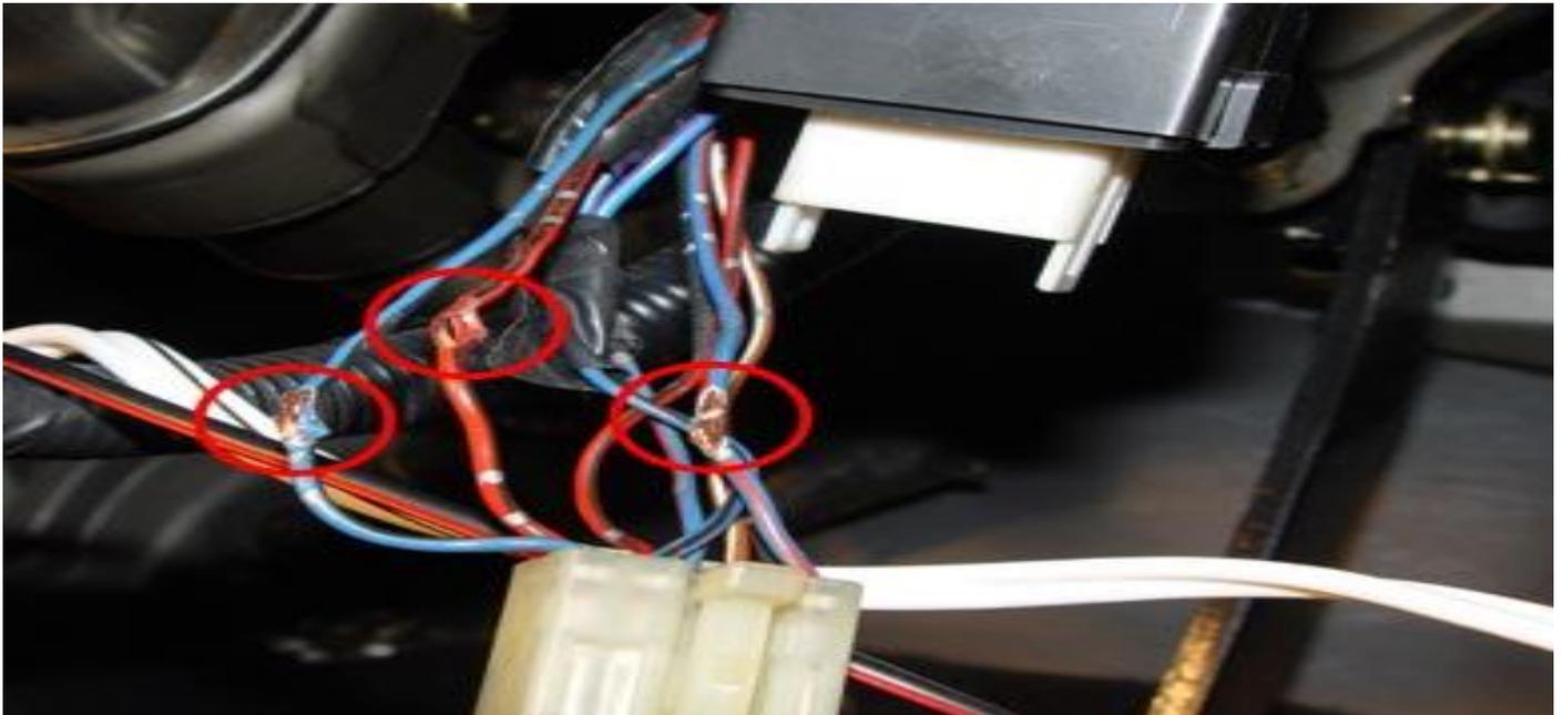
Pull the plastic connector out. Take a sharp knife and cut some of the insulation from the wires that go to pins 1, 3 and 8 as shown in the schematic below. You may prefer to use a connector which splices the wire for you.
