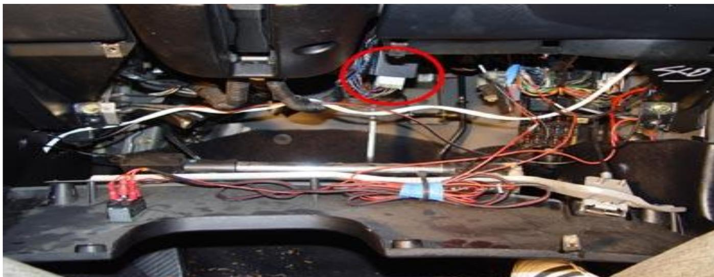
Remove the four screws and drop the panel under the dash. Locate the central locking control unit (circled in red).
