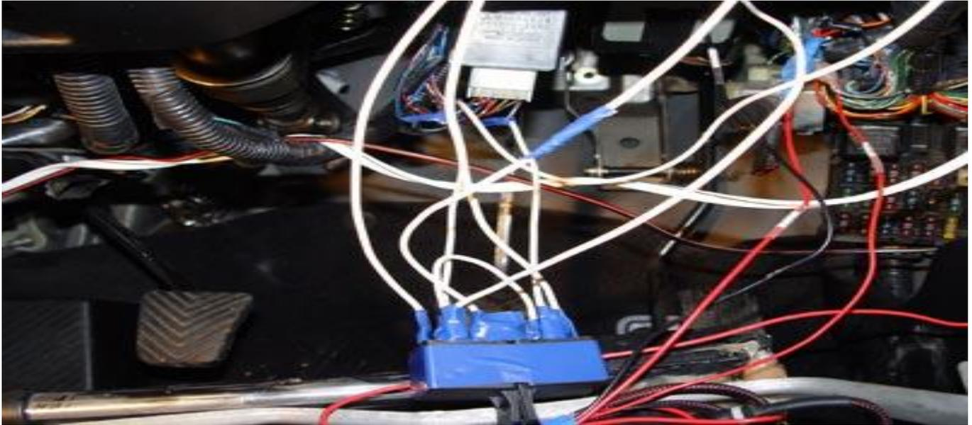
This part takes the longest but is relatively easy: Connect the relays following schematic v1.0 above. I taped both relays together back to back as you can see at the bottom of this image. There is a convenient ground point to the right of the central locking control unit.
