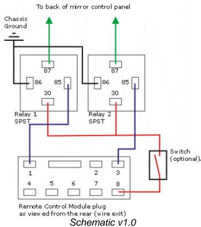
Schematic showing wiring connections - based on original by Tim M.
