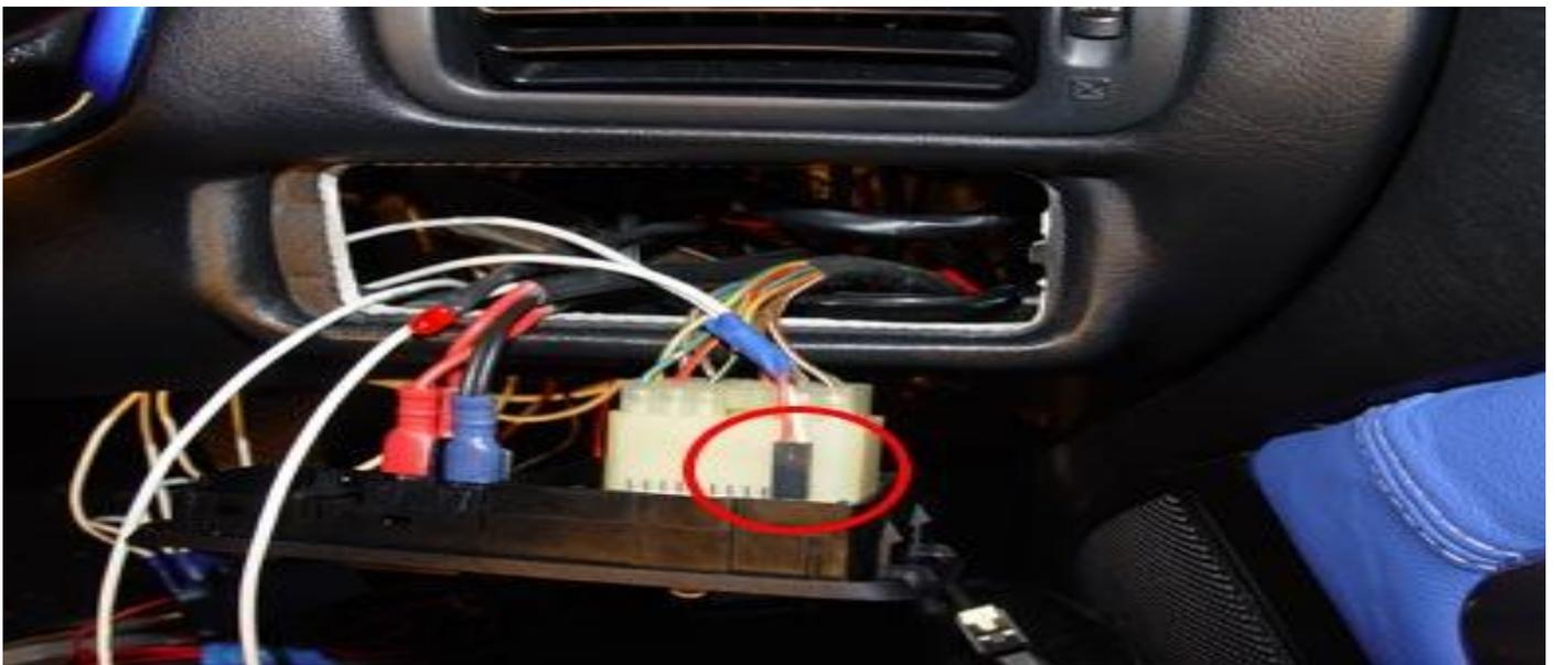
Remove the mirror control panel, lift up the black plastic cover to reveal the pin connectors and attach the open and close signal wires to the two rightmost pins. I used a pin connector from an old PC case instead of messy soldering here. Test the central locking and if the mirrors fold incorrectly (ie. fold out when car is locked then simply swap these two connections around).
