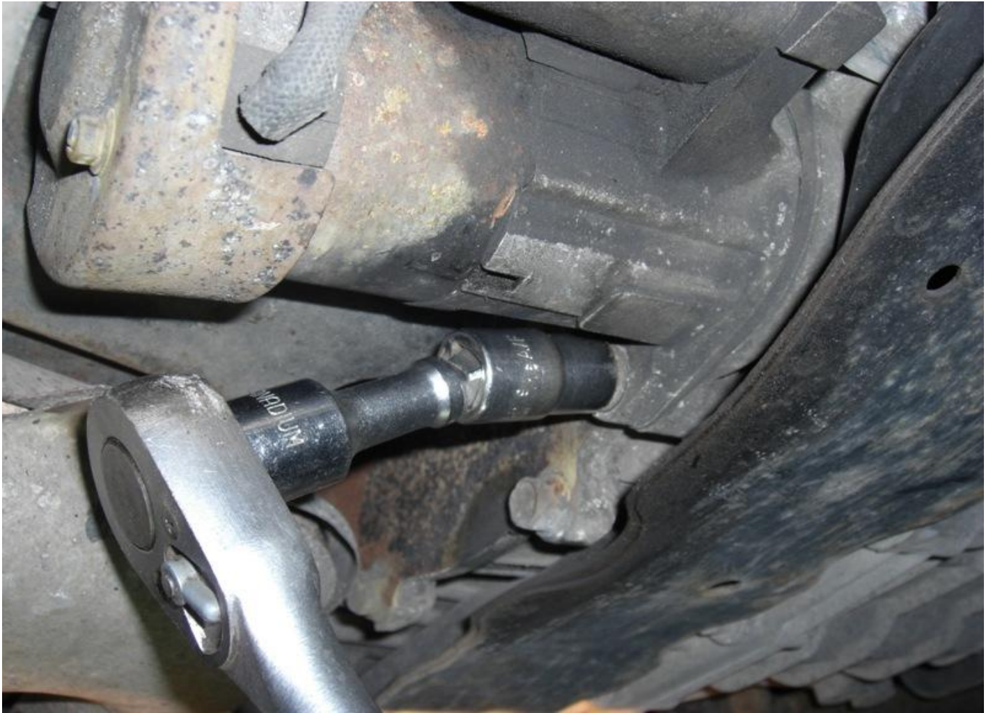
4) UNDOING THE OIL DEFLECTOR'S BOLTS
