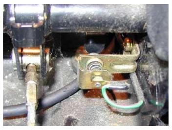
As you can see from this photo there gathers alot of crap under here. Clean the plunger and oil it slightly if required. Check the contact of the green wire, and bend the bracket slightly forward to get a better movement of the lever. Test it a few times to make sure the light goes out. If it does, you're sorted, if it doesnt it may be something more serious to do with your brakes and you should ask a mechanic.
