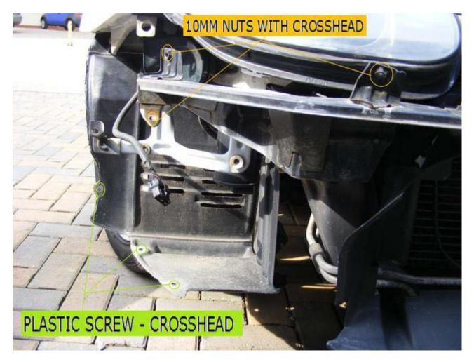
undo the plastic screws along the top of the bumper (in between the headlamps), pull the bumper forward under the light and another 2 screws (either side) will show themselves for you to unscrew, the metal flanges securing the bumper at these bolt points will also bend but dont worry as after market bumper dont use these bolts hole (my facelift t's factory facelift didnt use these) the flange can easily be bent back with pliers or a hammer.
