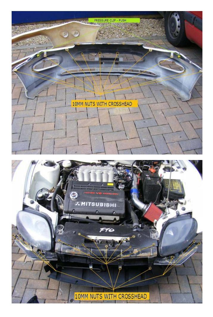
finally slide your arm down the inside of the centre bumper to undo the 3 screws located at the top of the grill and the bumper will come away.
