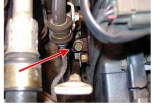
Using a socket set turn the bolt clockwise and you'll notice the adjacent fanbelt pulley begin to rise. Check the belt tension and adjust as necessary.
