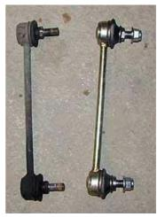
front hub. It is held on with 2 nuts which you need to remove. The threads do get badly corroded so you may have to resort to sawing the nuts off but you may not have to if you're lucky. You might also have to use the breaker bar to initially move them. Dont worry about sawing them off though, because the washer saves damage to the mounts and your new droplinks come with nuts (or at least they should do!).
