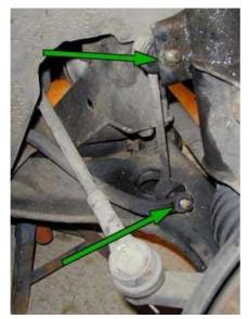
Undo the nuts using the spanner (14mm I think) at the back between the ball joint and the mounting to stop the droplink revolving. There's a slot for it to fit into (check the new one to see what I am talking about here).
