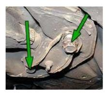
It now gets tricky. You need to remove a 12mm bolt which secures a cup over the bush. To do this, you need to lever down the suspention arm while putting the spanner around the back. You'll only be able to move the bolt 1/8th turn at a time, but percivere and it will work.
